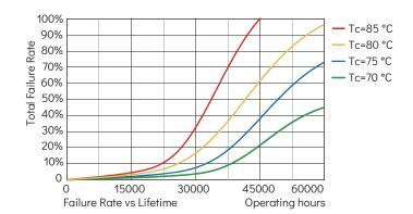
Lifetime estimation based on the application environment condition: at room temperature (25°C@ 10mm free air), base down burning position, and at rated voltage.
